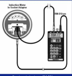
Running a test using an RM-DS/sm Suction Mount Disk Sensor
